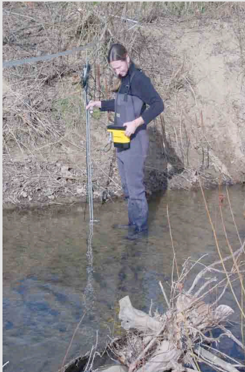
Velocity Measurements recorded using an Electromagnetic Flow Meter
