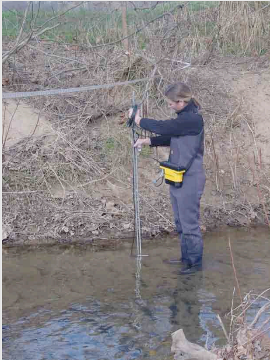
Velocity Measurements to Estimate Discharge
